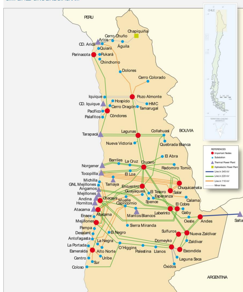
SIMPLIFIED SINGLE LINE DIAGRAM
